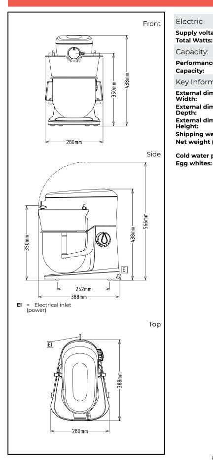
Electric Supply voltage: 200-240 V/1N ph/50/60 Hz **Total Watts:** 0.5 kW Capacity: Performance (up to): 0.75 kg/Cycle Capacity: 5.5 litres Key Information: External dimensions, Width: 280 mm External dimensions, 388 mm Depth: External dimensions, Height: 438 mm 15 kg **Shipping weight:** Net weight (kg): ISO 9001; ISO 14001 0.75 kg with Semi spiral **Cold water paste:** hook
